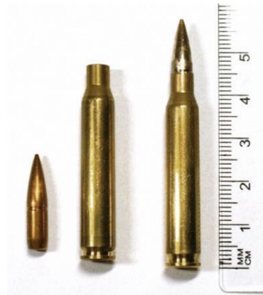
Figure 2 Modern bullet 5.56mm in diameter. Left to right: Bullet, case and complete cartridge. [9]
